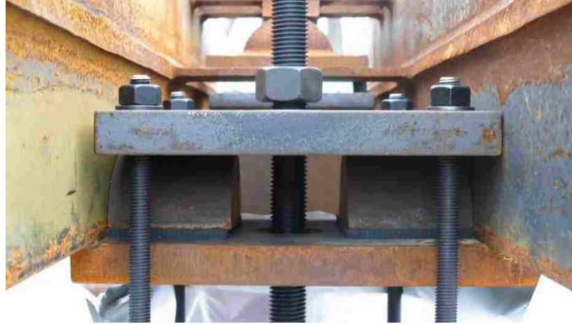
(a) Snug four small top nuts and loosen Nut B
