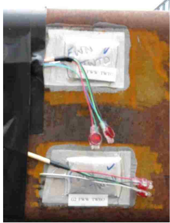
(b) Uniaxial strain gages on girder tube
