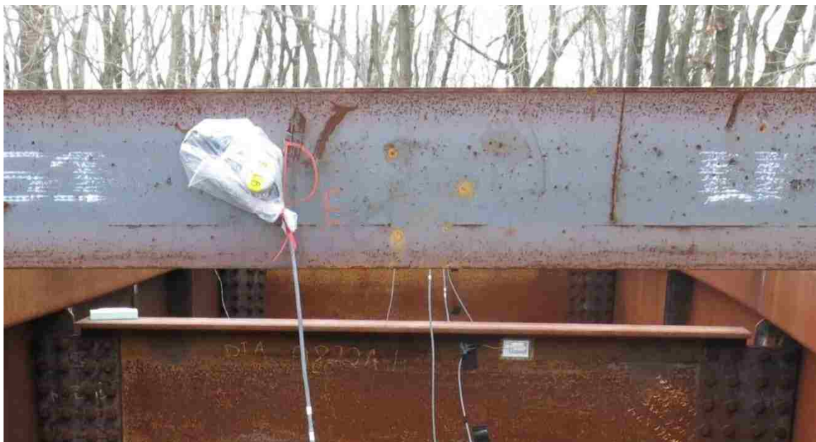
(c) Inclinometer attached to loading beam to measure rotation in parallel plane
