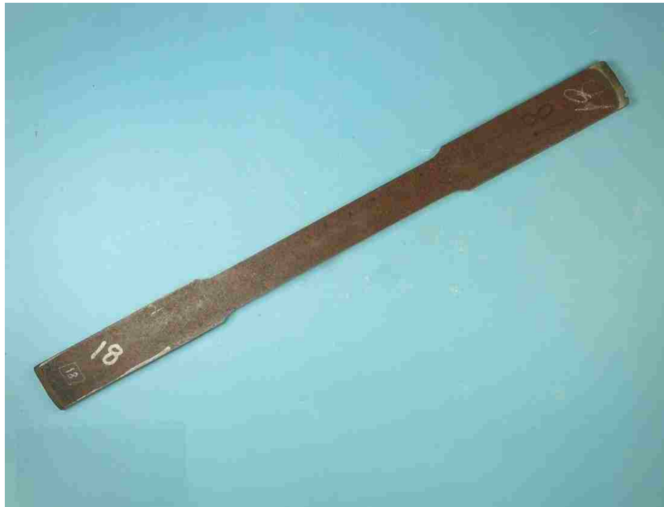
Figure 8.7 Plan view of typical tensile coupon
