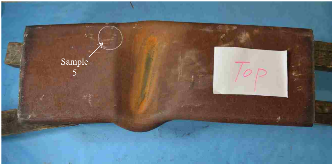
Figure 8.15 Buckled section looking from top
