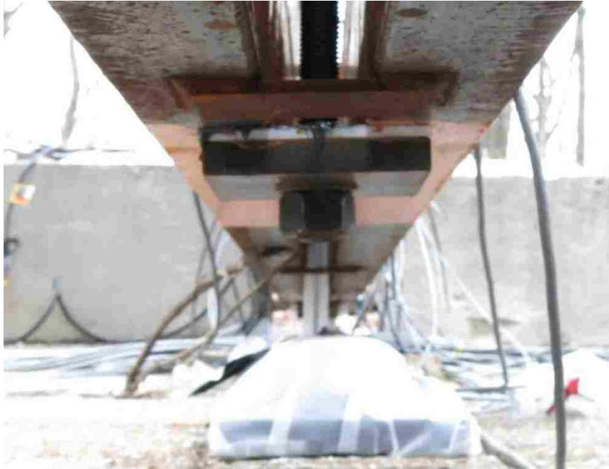
(a) Photograph of bottom of loading rod assembly looking in parallel direction
