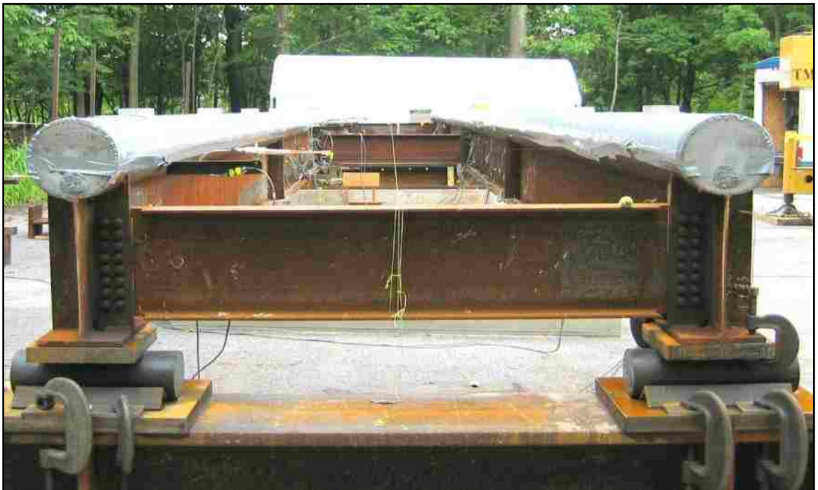
Figure 2.2 Straight TFGs with concrete-filled round steel tube top flange (Kim and Sause, 2005a, b)
