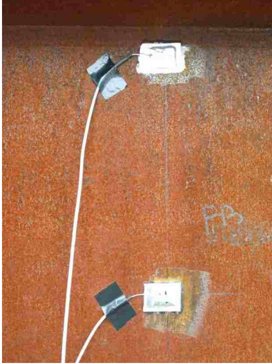
(a) Bending moment full bridge strain gages on girder web
