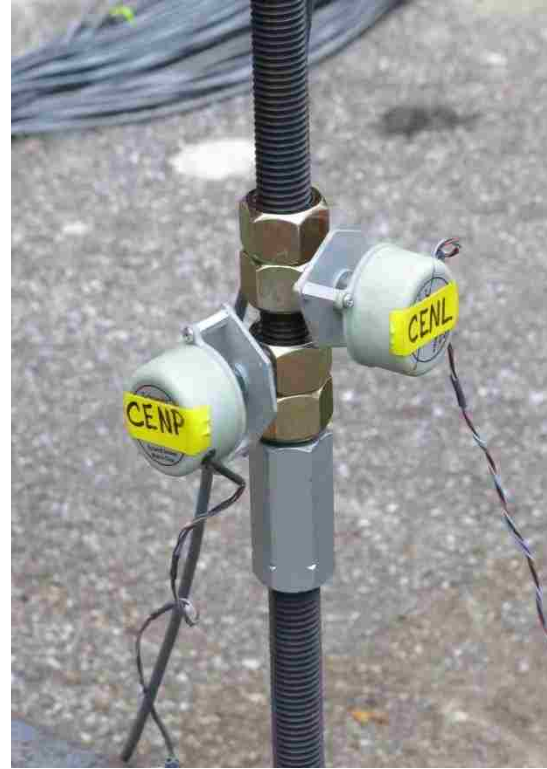
(b) Inclinometers attached to loading rod to measure rotation in parallel and longitudinal planes
