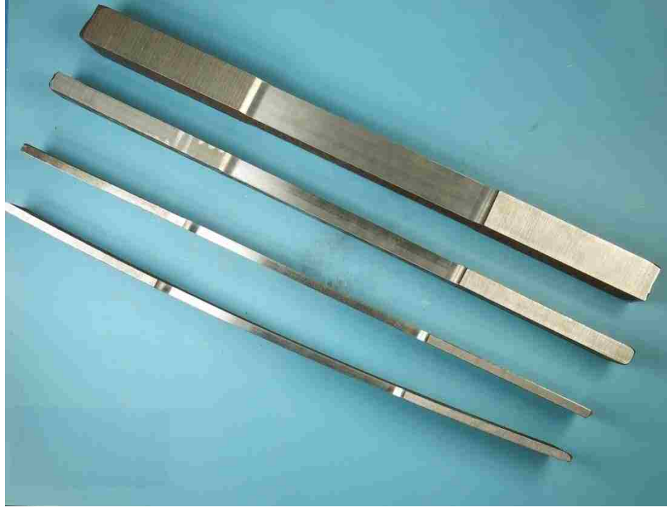
Figure 8.6 Side view of tensile coupons (from top to bottom: G2 bottom flange, G1 bottom flange, G2 web and G2 tube)
